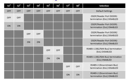
Both DIP Switch 7 and DIP Switch 8 need to be either On or Off to be properly configured.
