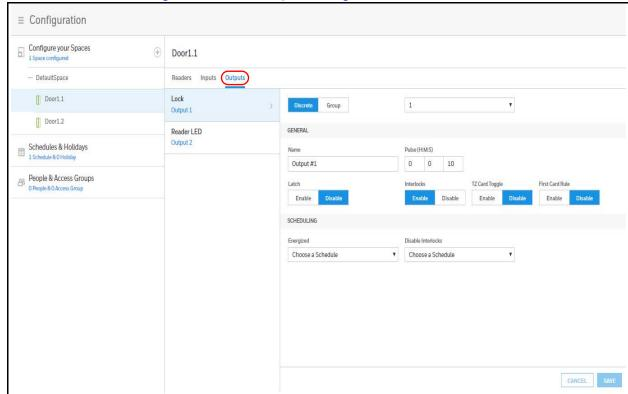
Figure 3-6 Door Outputs Configuration Interface
