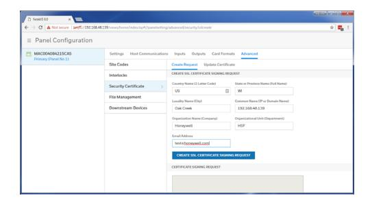
Go to **Advanced Menu > Security Certificate** tab. **Create Request** will be selected at the top of the pane. Fill in the fields as shown above. Make sure that the panel IP address is in the common name field.
