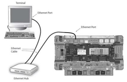
b. Web server direct connection: Connect the computer's Ethernet port directly to the panel's Ethernet port with either a crossover or an Ethernet cable.
